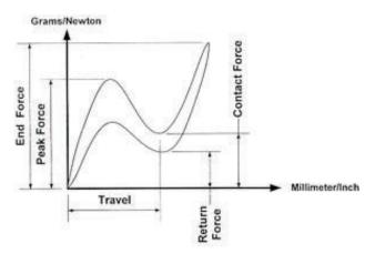
Above shows a typical force curve displacement when a knob of a keymat is depressed.
